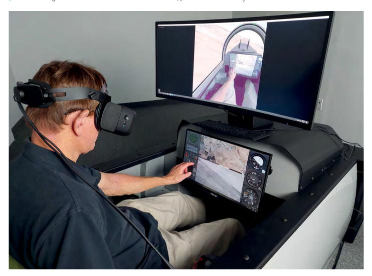
**Above**: The PTMT can be networked to function as an additional aviation role-player station as part of the DJFT, or function as the Aircrew station.
