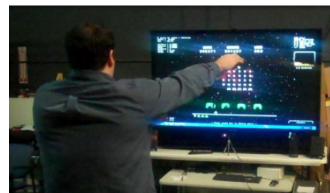
Figure 5. User controlling a standard game with gestures through keyboard emulation option in FAAST
